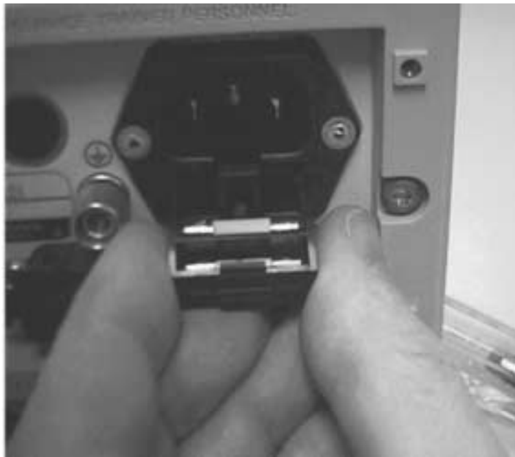
Figure 6. Replacing Fuse Holder
